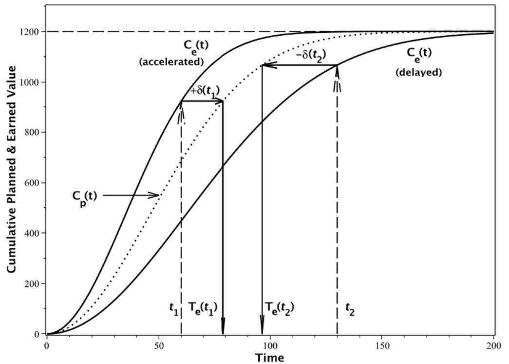
Figure 2 Definition of the delay,  $\delta(t)$ , as the difference between the earned and planned value curves:  $+\delta(t_1)$  is an accelerated project, and  $-\delta(t_2)$  is a delayed project. The corresponding earned durations are denoted as  $T_e(t_1)$  and  $T_e(t_2)$ .
